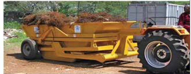
Figure 7.31 A very simple winch-on system can be used as a container lift or a conventional trailer
