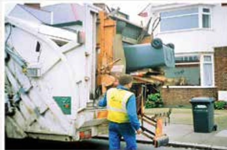
Photo 7.19 Compactor truck with binlift
