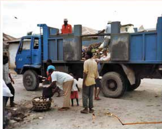
Photo 7.10 High-sided vehicle with side doors to assist loading
