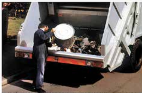
a) The low loading height and large hopper are big advantages
