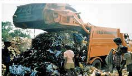
b) The waste is pushed out hydraulically by the compression (or ejector) plate
