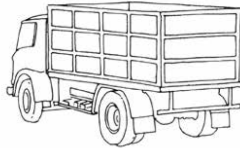
Figure 7.11 High-sided open top vehicle
