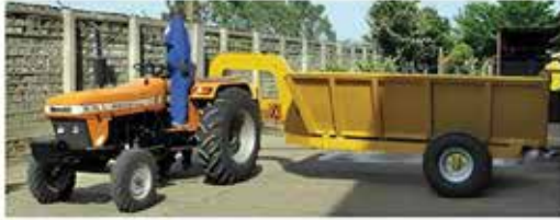
Figure 7.9 Swan neck trailer drawbar greatly improves manoeuvrability
