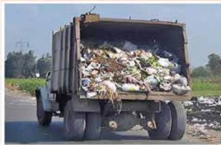
Photo 7.20 When the compaction mechanism cannot be repaired it can be taken off
