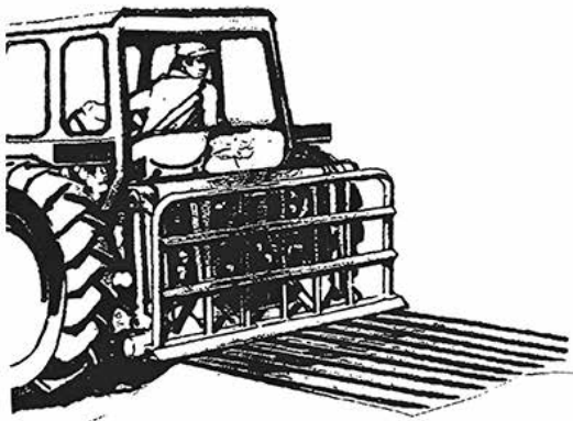
Figure A5.2 The agricultural buckrake for spreading wastes
