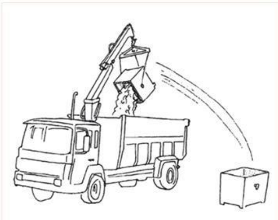
Figure 7.17 Crane system reaches out to pick up containers
